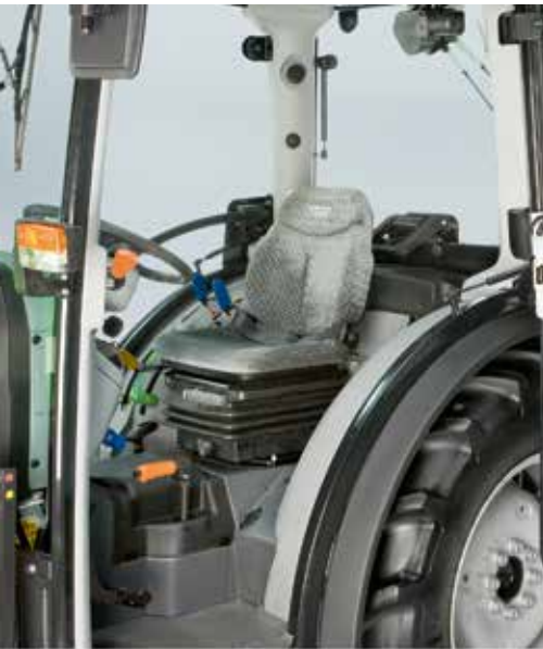
Mechanical or air-sprung comfort seat.
