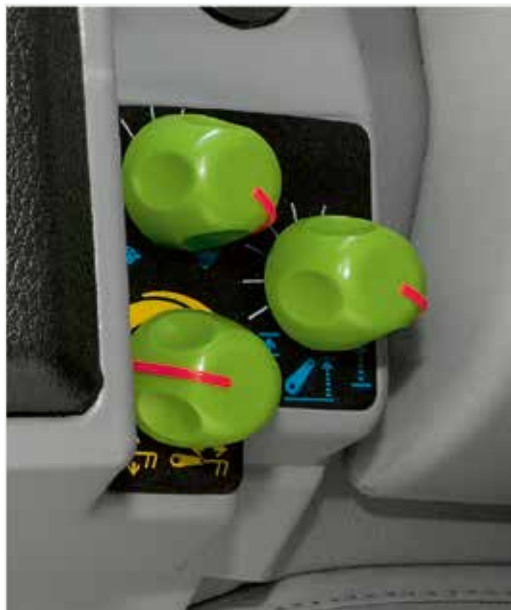
The Electronic Hitch Regulation can be adjusted quickly and easily with rotary regulators.
