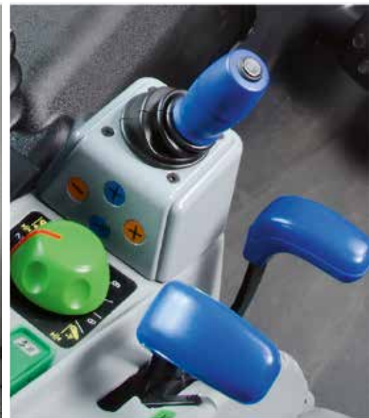
Joystick operation of the additional remote valves upon request.
